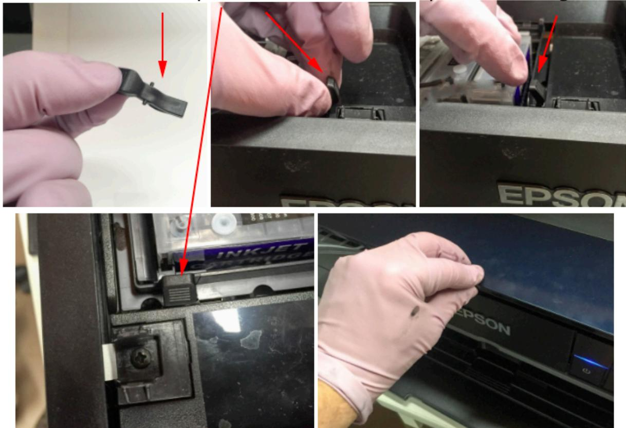
**Printer Cover Switch:** There is a second small switch provided with your ink set or cartridge. This second switch tricks the printer into thinking the entire printer cover is still down. Put this switch deep into the middle slot of the printer (just to the right of the first switch) as shown on the right. It will lock into place. You can keep this switch in forever.
