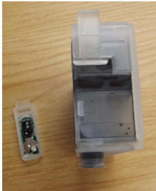
2. Note the plastic chip base has two prongs on top. To attach a new chip to the cartridge, slide these two tabs into the channels under the cartridge locking tab as shown below, then press the bottom of the chip onto the cartridge so it snaps into place and is flat on the cartridge.
