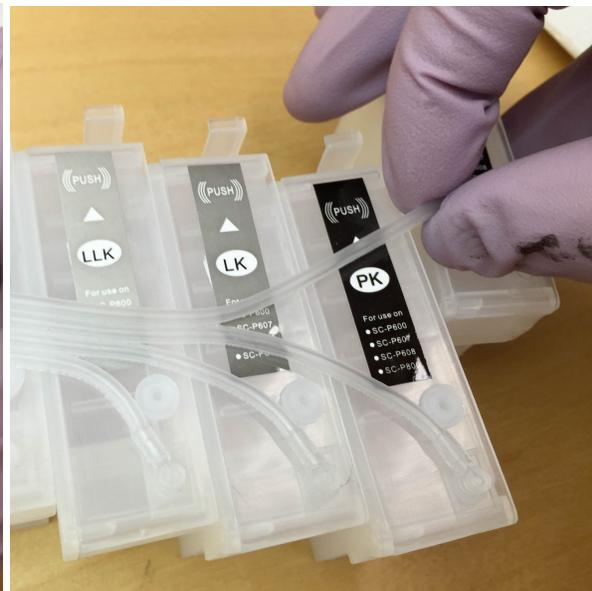
6. Rotate each ink inlet about 90 degrees as shown below. This will allow the ink lines to exit the printer at the right angle without restricting ink flow (very important).
