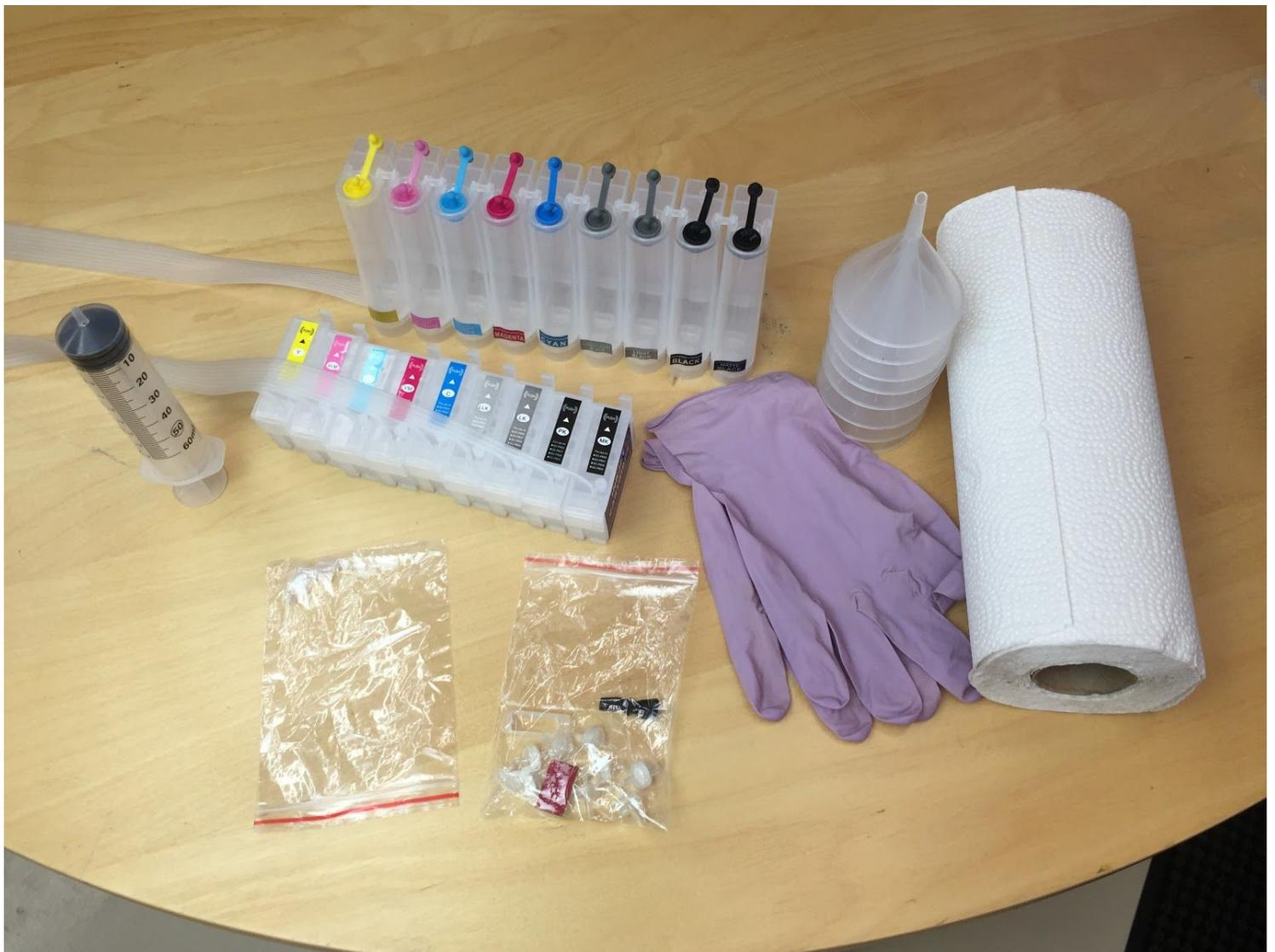
3. Take out your ink and identify which ink bottle will be poured into which CIS tank. The tanks have small stickers at their bottom that marks the ink-shade they are designated for. ConeColor Pro inks are easy, just match each bottle with each ink-tank.
